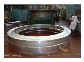
**Bulkhead for Fuel Tank Bottom Dome**
