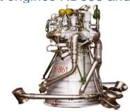
Upper-stage rocket engines with multiple restarts (RD861)
