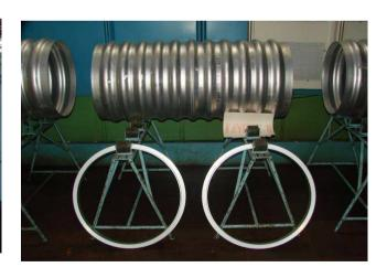
Fuel Tank Tunnel Pipeline (for Oxidizer Feedline)
