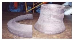
Nozzle extension for Solid-propellant rocket engine
