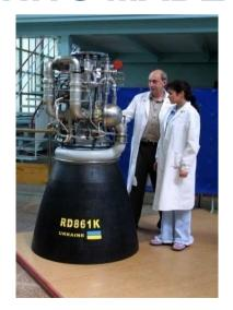
Liquid-propellant rocket engine with uncooled nozzle extenstion made of carbon-carbon
