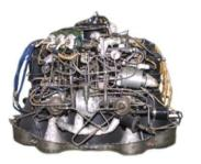
Lunar Landing Module liquid rocket engines RD858 and RD859
