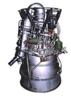
Rocket engines with gas-dynamic thrust vector regulation (RD862)
