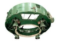
Steering engines for 1st and 2nd LV stages (RD8)
