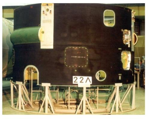
It is manufactured from aluminum alloy and has waffle structure.
